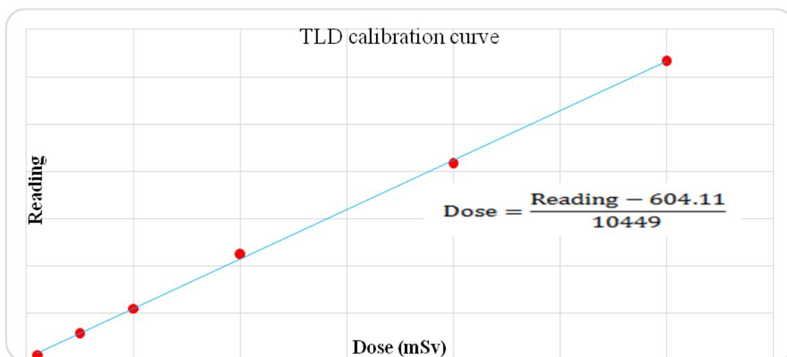
**Fig1:** TLD calibration curve
