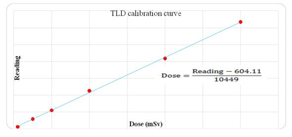
Fig1: TLD calibration curve
